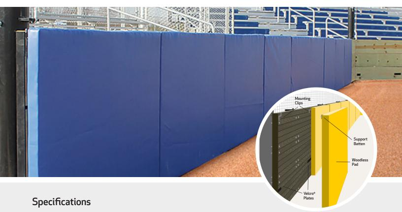
**Vinyl Covering:** 18oz./sq. yd. fully COATED vinyl on base fabric scrim of 1,000 denier x 1,300 denier polyester. Fabric meets following tests: Tear Strength Tests: Warp 100 lbs., Fill 100 lbs., Grab Tensile Strength: Warp 410 lbs., Fill 410 lbs., Weft Insertion: 18 x 17. Vinyl compounded with UV inhibitors and mold inhibitors. Cold Crack: Minus 40° F°.
